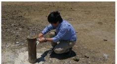
Water lever meter to monitor groundwater
